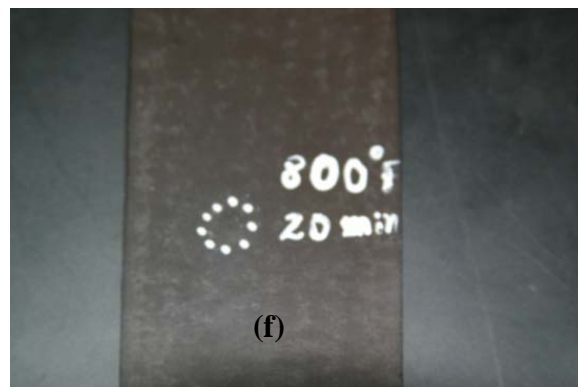
Figure 49. THz TDS images and photos for three burn areas on glass fiber samples: (a), (d) 440°C for 4 minutes; (b), (e) 430°C for 6 minutes; and (c), (f) 425°C for 20 minutes.
